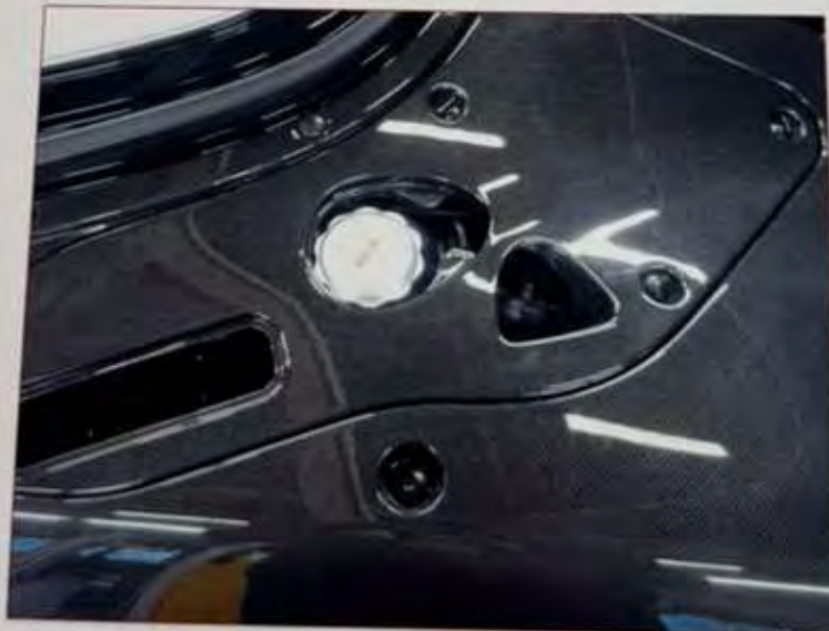
serbatoio olio Oil tank
